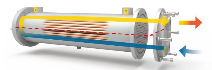
The hydraulic circuit with double passage leads to small dimensions with the same thermal performance. For easy installation, the cooling water inlet and outlet connections for the water-glycol mixture are located on the same side.
