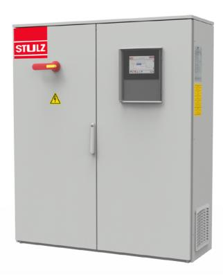
The switch gear cabinet is on the longitudinal side of the chiller and was generously dimensioned so that all deliverable options as well as customer-specific adaptations can be integrated therein. The components in the switch gear cabinet control the entire functional scope of the chiller. The switch gear cabinet has two or three doors, is ventilated and is equipped with a load-break switch including door blocking and a display for the controller.
